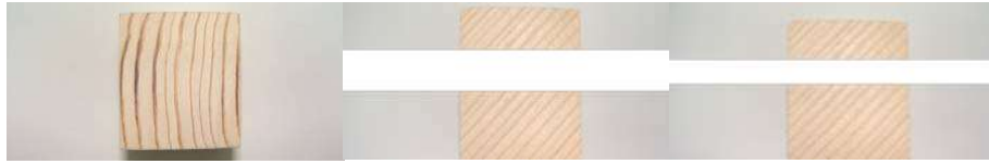
Fig. 3 – Debiting the wooden material perpendicular on the fiber, the fiber having an aesthetical role due to the game of tones and direction.
