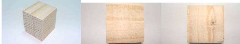
Fig. 4 - Debiting the wooden material longitudinal with respect to the wood fiber. The fiber presents an aesthetical role, through the game of colour tones, direction or some existent defects in the wooden structure (nods).
