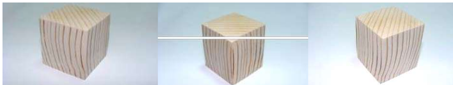
Fig. 2 – Debiting the wooden material perpendicular on fibber, the faces of the cube revealing the fibber in different ways on every face.
