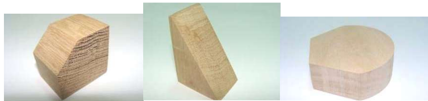
Fig. 5 – Different finishing types in wood (different tones, revealing the wooden structure in a different way, the quality of the surface, more or less shiny) are the result of cutting the different wood essences (lime, oak, etc.)
